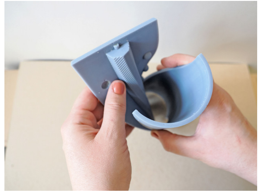
Above and on the previous page, The mould matrix made with an SLA printer and the silicone mould into for casting the wax.
