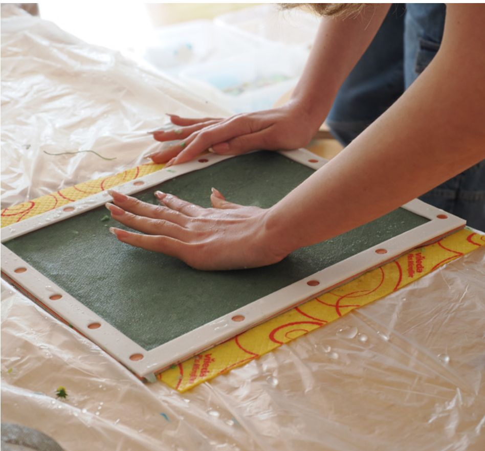
Above: the process of creating paper sheets with the 3d printed frame. Next: experimental prototypes and color tests in paper concrete.
