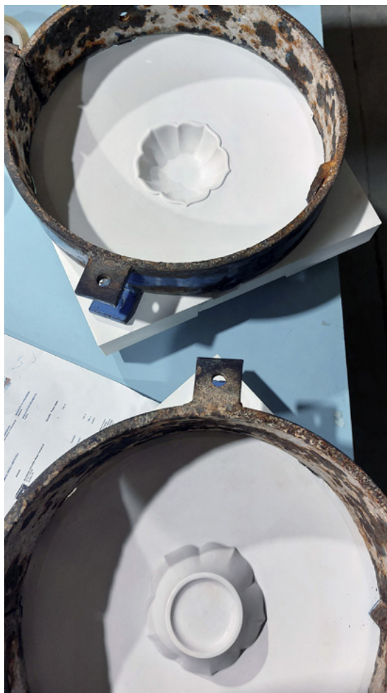
Above: photographic relief of the iron hoops. On the side: the hoops positioned over the two 3d printed matrix ready for casting the plaster mold. Next page: the two parts of the mold installed on the pressing machine. Below: the pottery plates created by the mold.
